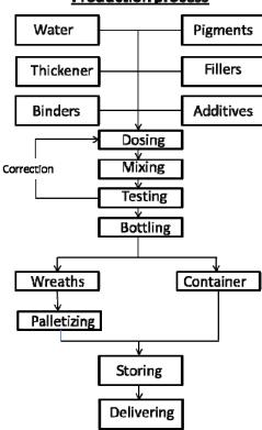
The figure shows the following working process during the production of external paint systems: First, the silos and weighting containers are filled, followed by transportation and adjustment of raw material into the mixer for dispersion. After a quality control, the external paints are filled into containers. Then they are loaded and delivered.
